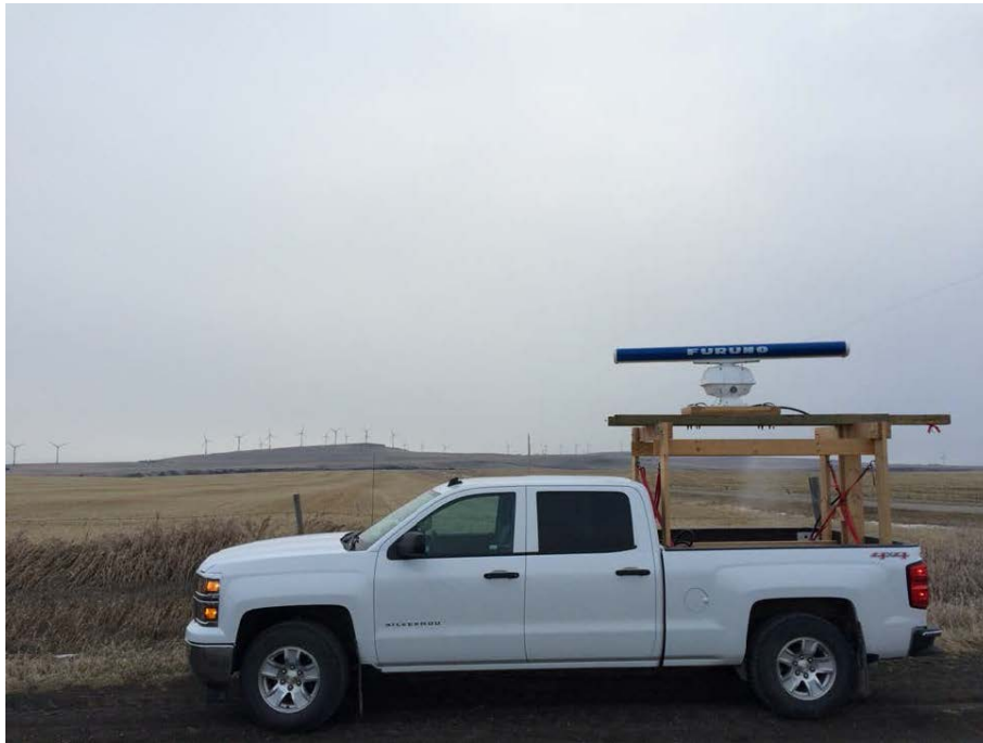
Photo 1 Truck-mounted marine radar unit used for nocturnal radar surveys
